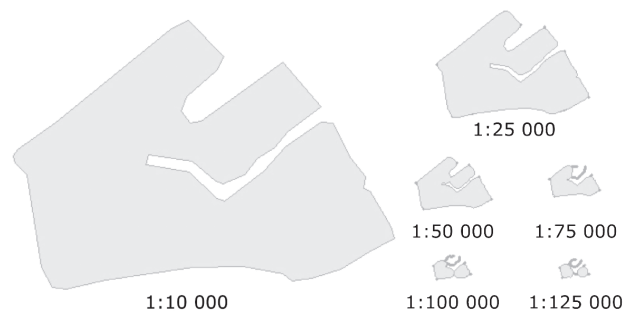
Fig. 8. Object “Mały Staw” generalized to 5 final scales. Presentations in all the scales are preserving the proportions
